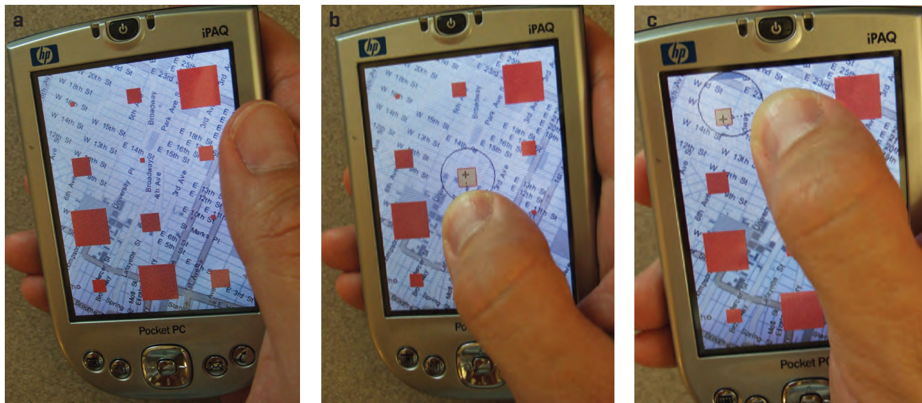
Figure 2: [a] Small targets are occluded by a user's finger. [b] Shift reveals occluded screen content in a callout displayed above the finger. This allows users to fine tune with take-off selection. [c] By adjusting the relative callout location, Shift handles targets anywhere on the screen.
