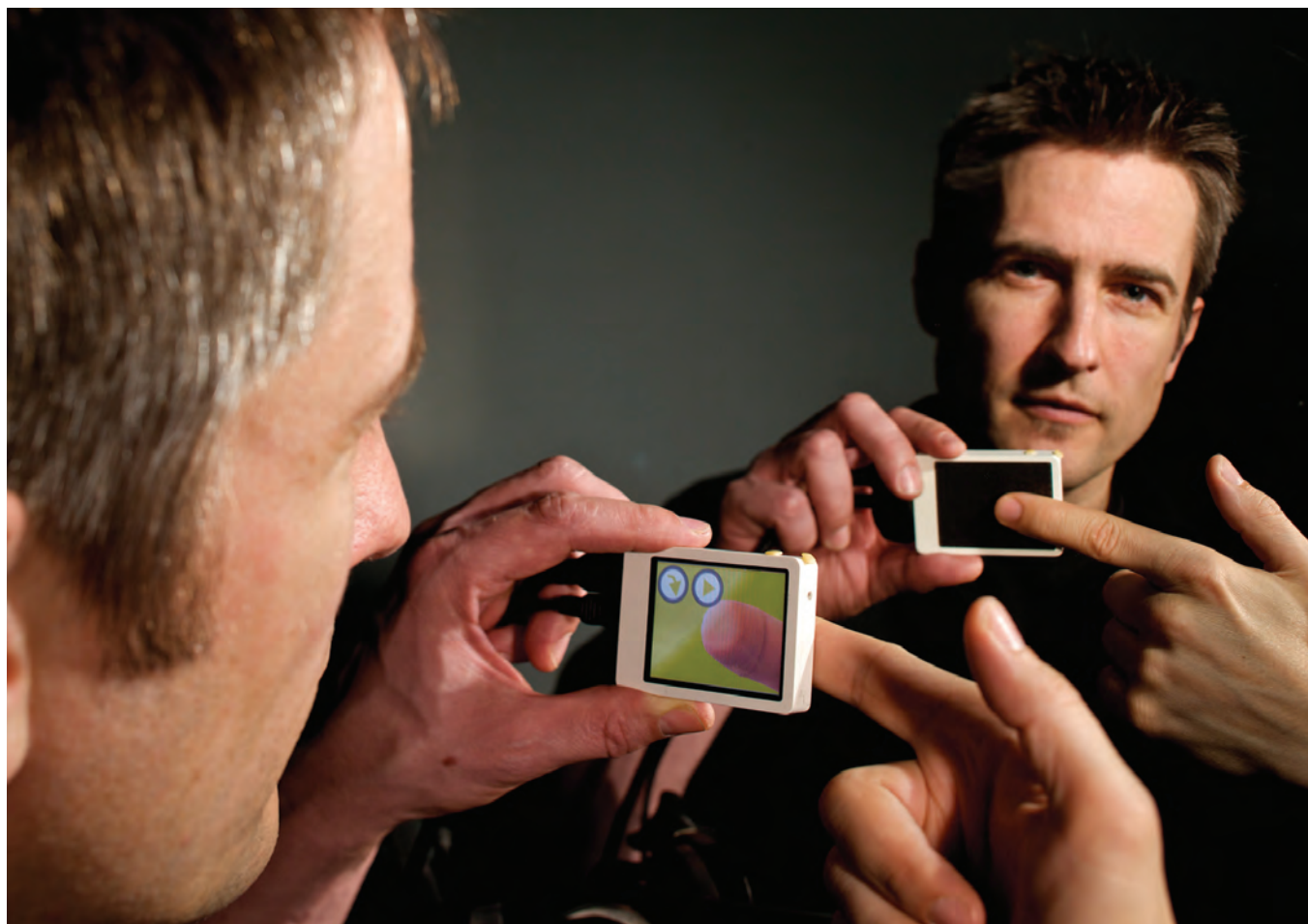
Figure 3: Users operate Nanotouch using pointing input on the back of the device.
