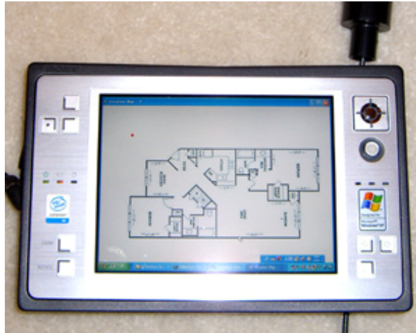
Fig. 4. User interface used for mapping and localizing the position of the connected receiver
