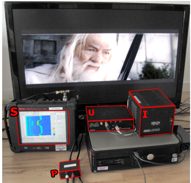
Figure 2: Components of our EMI capture hardware: Power Line Interface (P) for filtering 60 Hz signal voltage sensing, high speed digitizer (U) for analog to digital conversion of signals and an isolation transformer (I) for filtering EMI from other devices in our laboratory environment. The Sharp 42” LCD TV and the data logging PC are also visible. We also connect a spectrum analyzer (S) for debugging purposes and for visualizing the real-time EMI signal as a waterfall plot.
