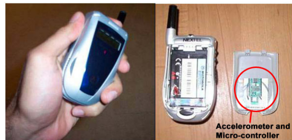
Figure 1: Prototype of a Motorola i95cl instrumented with a 2-axis accelerometer.
