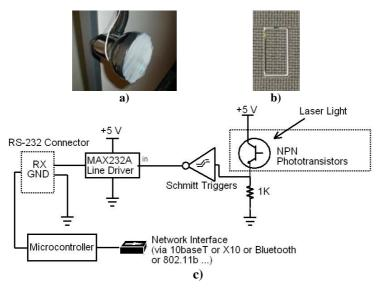
**Fig. 2.** a) A cone-shaped light-sensitive tag. b) A layer of phototransistors replacing a wall plate for a light switch shows a different form factor for the active tag. c) The schematic for the active tag.
