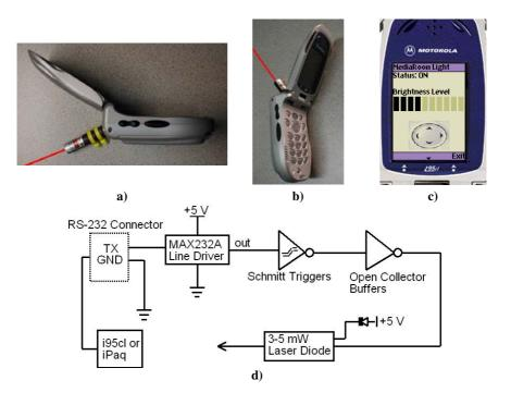
**Fig. 1.** a-b) The instrumented cell phone handset, a Motorola iDEN i95cl. The antenna is angled slightly to accommodate reading the screen while pointing the laser. c) A simulator screen for the phone showing a simple control screen for an X10-controlled light switch identified through laser interaction. d) A schematic for the laser controller.
