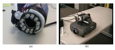
Figure 3. On the left shows our camera detector unit. We outfitted a Sony HandyCam, placed in *NightShot* mode, with a collection of IR transmitters and covered the lens with a narrow bandpass IR filter. On the right shows our camera detector coupled with a projector to neutralize cameras in the environment.
