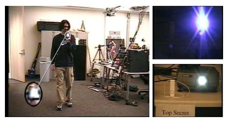
Figure 5. The left shows a camera phone being neutralized by our system (notice the neutralizing light beam over the lens). The top right shows the camera view neutralized by the system, the bottom right shows the camera view when the camera is permitted to capture the view.
