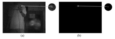
Figure 2. On the left, an unprocessed IR view captured by our camera detector with plenty of ambient light in the room. A person holds a camera phone pointed at a region in the environment we want to protect from capture. On the right is the processed view. The camera is detected by locating a bright white circular speckle.
