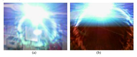
Figure 4. Images taken from a camera hit by localized light beam emitted by our camera neutralizer. The picture on the left shows a localized light beam generated using a single color. The picture on the right shows a localized light beam generated using color patterns that do not allow the cameras to adjust to the light source (notice the scan line).
