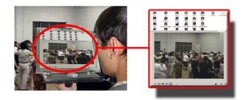
**Figure 6:** The ContextCam showing some live metadata (who and where) currently in the scene while capturing. The upper portion of the screen shows a thumbnail and name of each person currently in the view of the camera.
