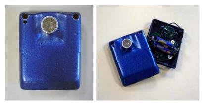
**Figure 3:** An active tag used to determine individuals in the view of the camera. A production tag could be much smaller and aesthetically pleasing.
