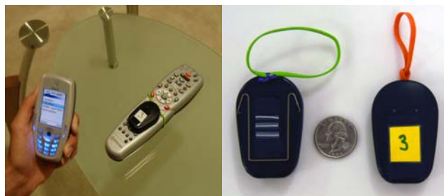
Figure 1: Left: User locating television remote control with phone. Right: Front and back of tags with a U.S. quarter to show size
